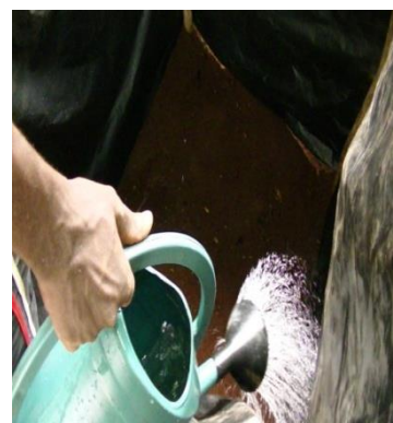
Photo 1c: 0.5m 3 pit with watering system
