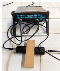
Fig. 3. Non-destructive dynamic modulus of elasticity method
