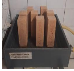
Fig. 4. Capillary water absorption of CEB
