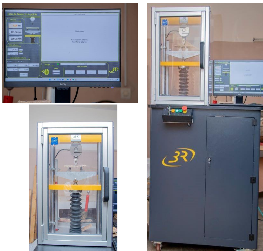
Fig. 4. Press for three-point bending tests
