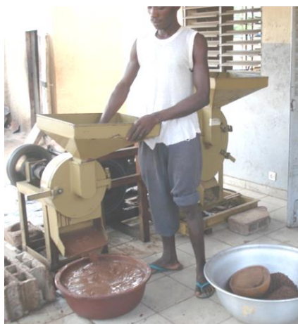
Fig. 9. Shea almond mill with carborundum stone
