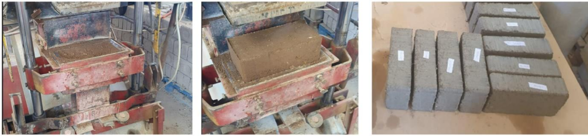
Fig. 3. main steps in the production process of CEBs, including 1. the filling of the mold 2. the block after compacting stress, and 3. Produced CEBs
