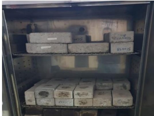
Fig. 4. Cured CEB samples in the oven
