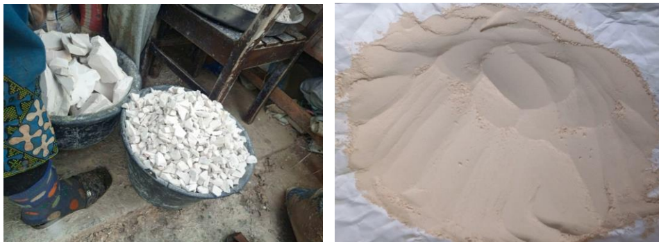
Fig. 4. Kaolin before and after calcination
