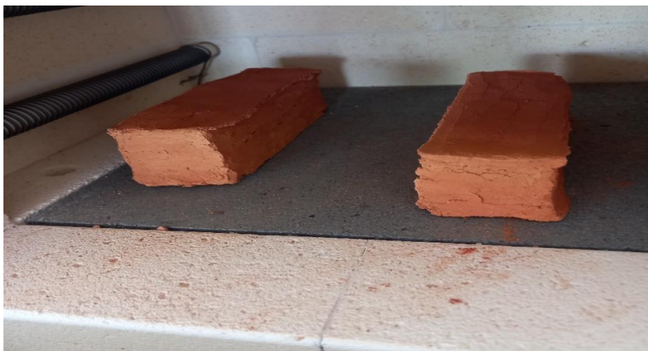
Fig. 8. Internal view of the oven after the test tubes have been fired
