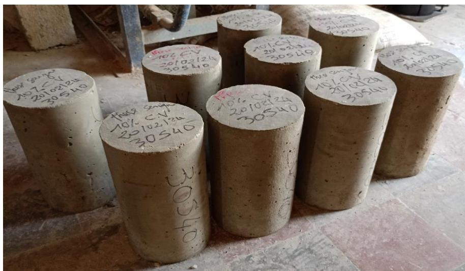
Fig. 3. Improved hydraulic concrete specimens, just after demolding
