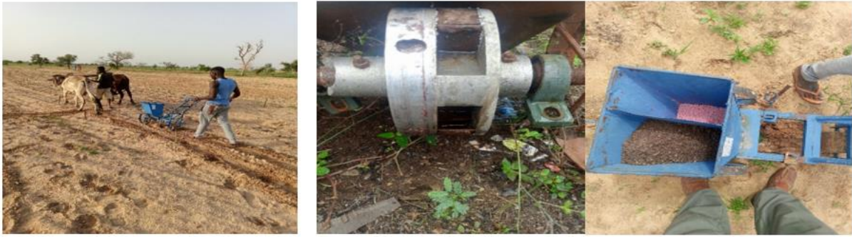
Fig. 1. The Gangaria Seed Drill: Integrated Tool for Simultaneous Sowing and Organomineral Fertilization
