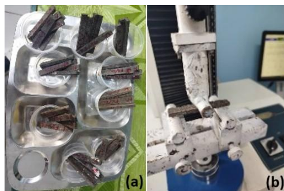
Fig. 6. Three-Point Bending Test (a) 3-point bending test samples (b) Sample on the machine
