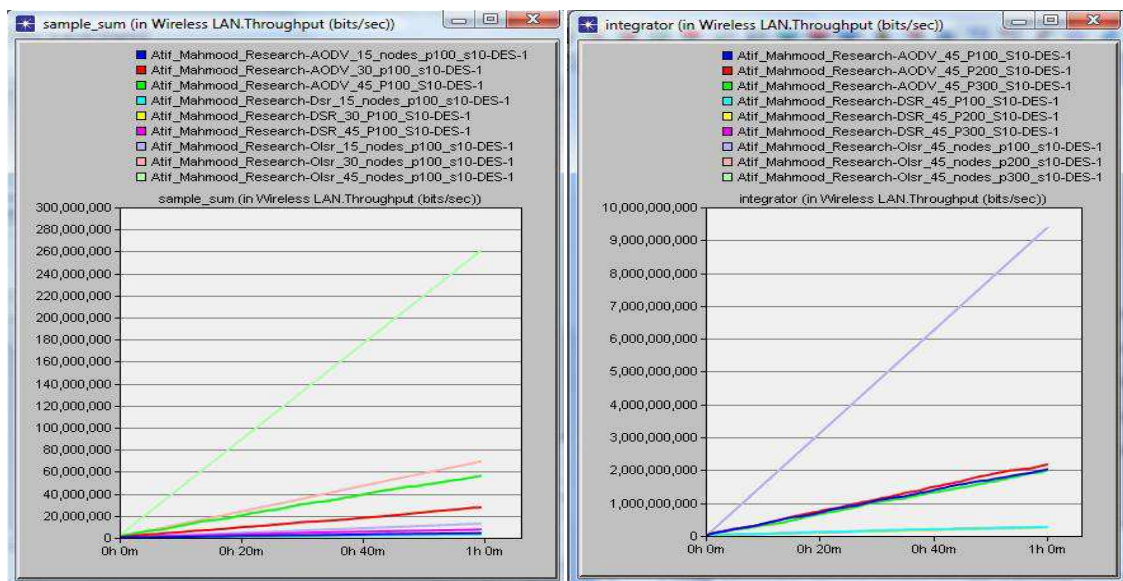
Fig 4, 5: OLSR, DSR and AODV Throughput vs pause time and no of nodes respectively
