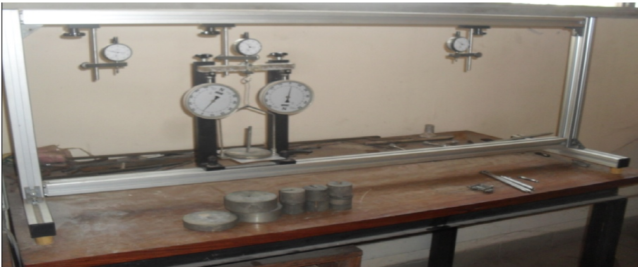
Fig.1: testing machine "3 point" bending
