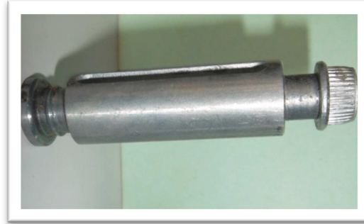
Plate 2: Machined specimen for wear test
