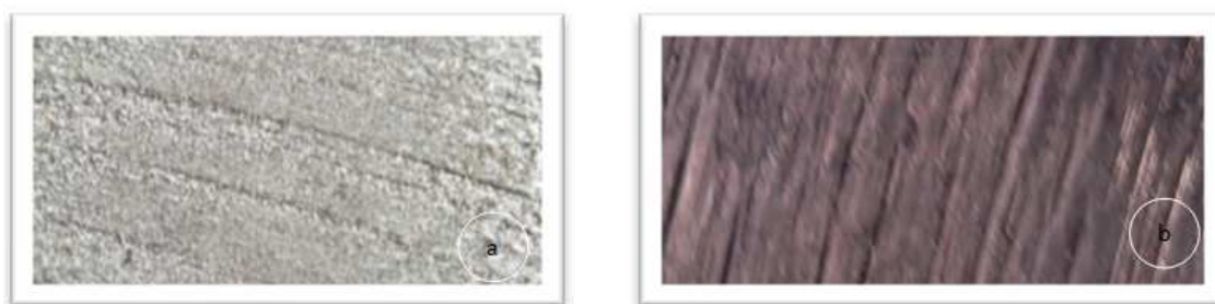
Plate 8: Machined as-cast surface after wear tests (a) with oil and (b) without oil
