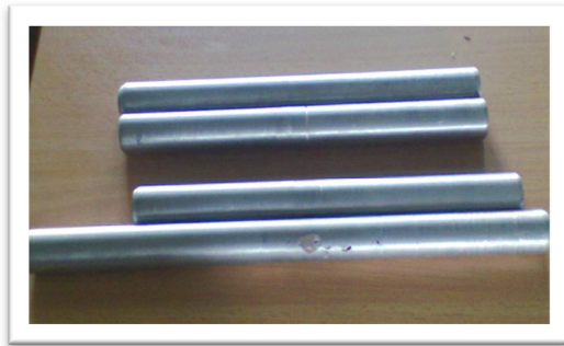
Plate 1: Turned cast aluminium alloy
