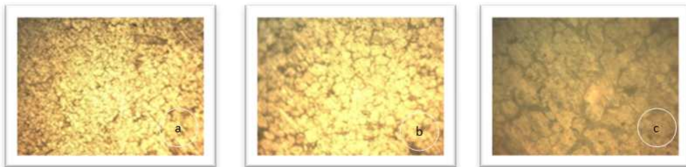
Plate 4: Micro-structure of As-received aluminium alloy sample
