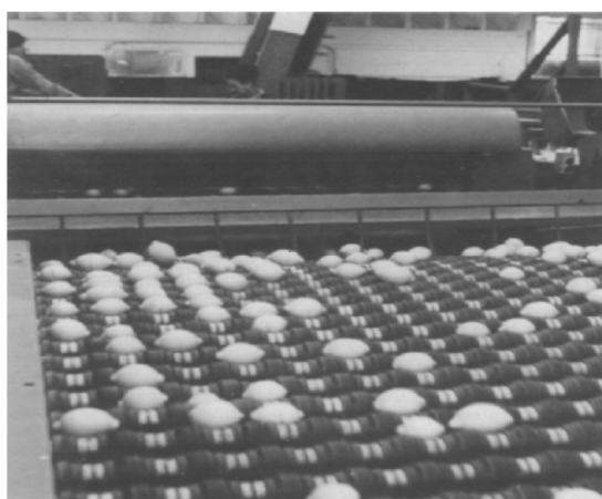
Fig. 1.1.5(b) Sorting lemons on a roller sorter.
