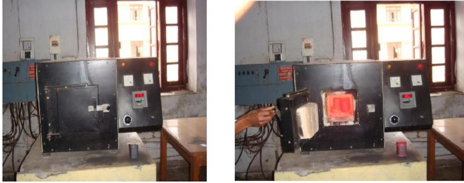
Fig. 1 Muffle furnace for carburization of mild steel samples
