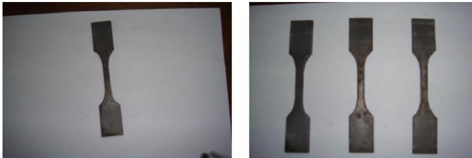
Fig. 5 Specimen for toughness test
