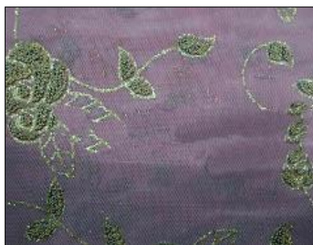
Fig.18. Foil Printing On Tulle Fabric
