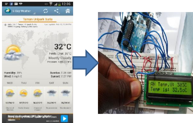
Fig. 2. Temperature calibration between android application and Robot temperature sensor
