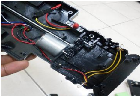
Fig. 4. Motor and gear system for the hind wheels
