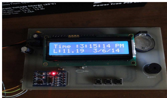
Fig. 11. Earthquake Detected by the Accelerometer
