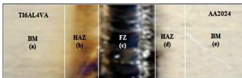
Fig. 5. Various zone at weldment both Ti/Al sides
