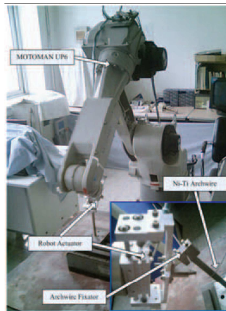
Figure 3: Archwire bending robot based on MOTOMAN UP6
