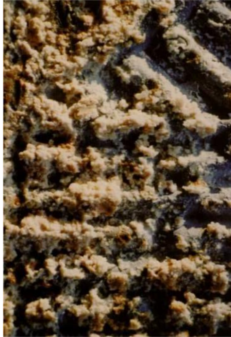
Fig. 1. Crystalline Fouling on a Plate and Frame Exchanger
