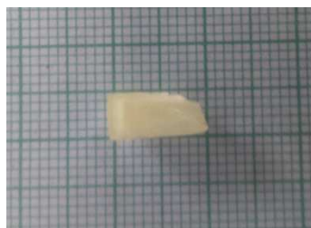
Fig. 2. As grown crystal of DNCB
