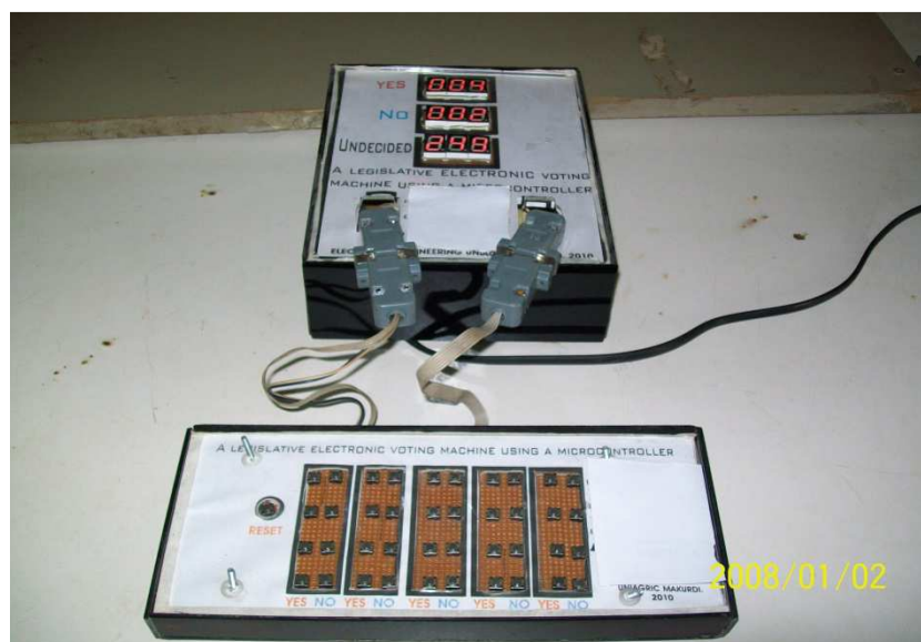
Fig. 9. The Legislative Voting System showing the Voting and Display Units
