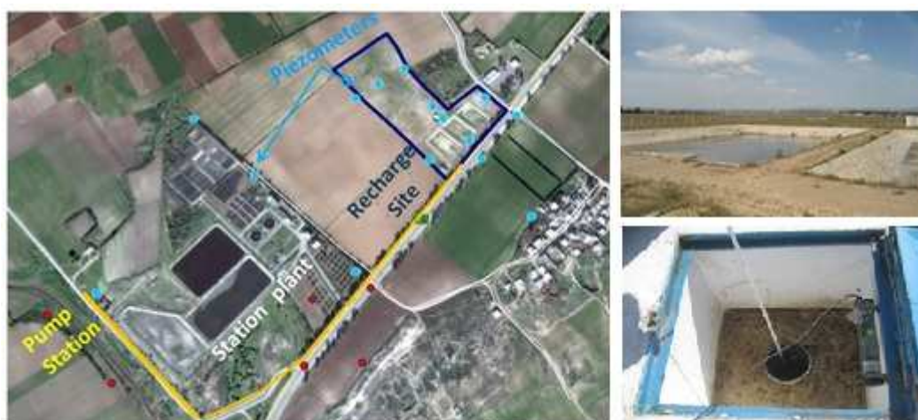
Fig. 4. Satellite image obtained from Google Earth showing the treatment plant and the recharge site, Picture during the filling of infiltration basins with TWW in recharge site and one of control piezometer
