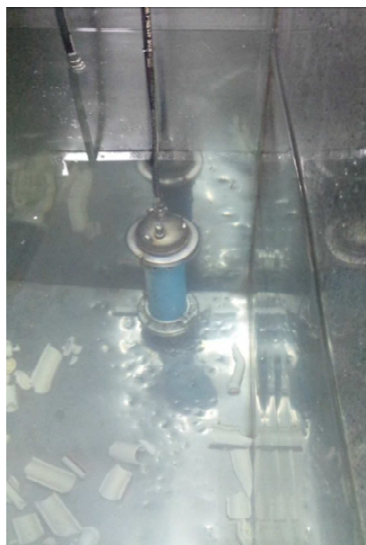
Fig. 4. Pipe immersed in the tank
