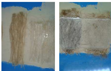
Fig 3.9 Working process of fibres a) applying of resin in the tray b) mixing of fibres with the resin c) adding layer of resin
