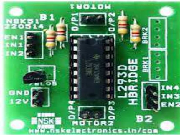
Figure: 10 H Bridge with different ports
