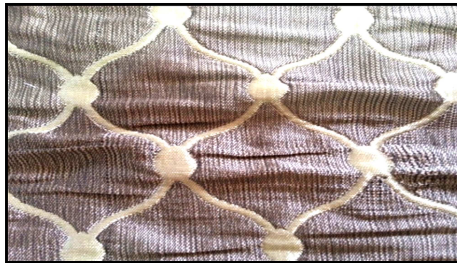
Fig. 13. The fourth sample which produced by warp tension variation method.
