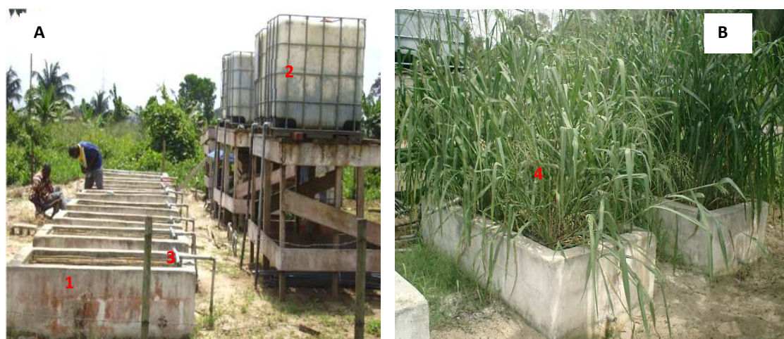
Fig. 1. View of the experimental device (A) and the vertical completely drained beds planted with P. maximum (B); 1: bed, 2: irrigation device, 3: feeding tank, 4: P. maximum growing on the beds.
