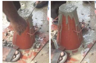
Fig. 1. Subsidence test in progress
