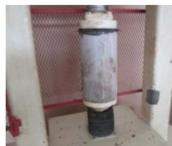
Fig. 2. Start of compression test on hydraulic press
