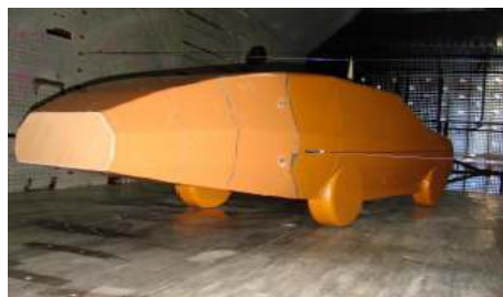
Fig. 8. SUV model with rear fairing [31]
