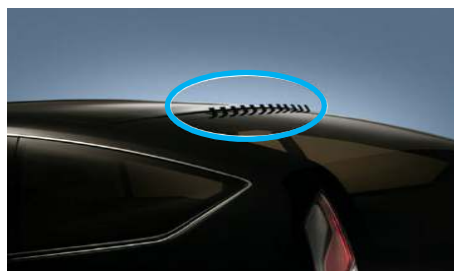
Fig. 4. VGs installed on the edge of generic car [31]
