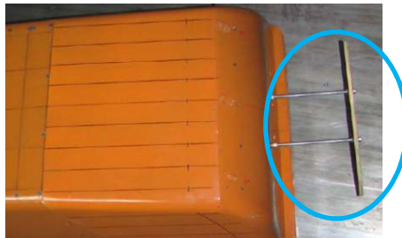
Fig. 7. SUV model with rear screen [31]
