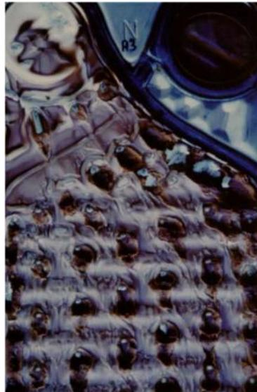
*Fig. 2. Reaction Fouling (Protein Deposition) on a Plate and Frame Exchanger Plate*
