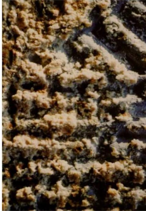
**Fig. 1. Crystalline Fouling on a Plate and Frame Exchanger**
