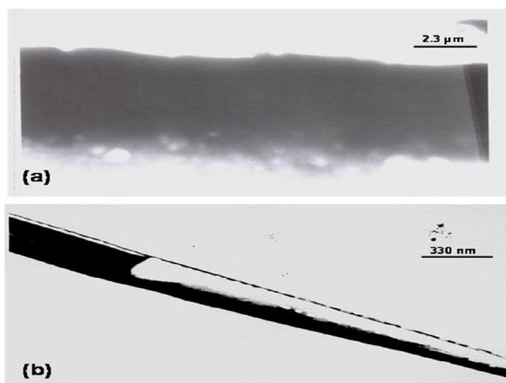
**Fig. 3.** TEM image of nanorods using (a) In the absence of catalyst (b) In the presence of catalyst.
