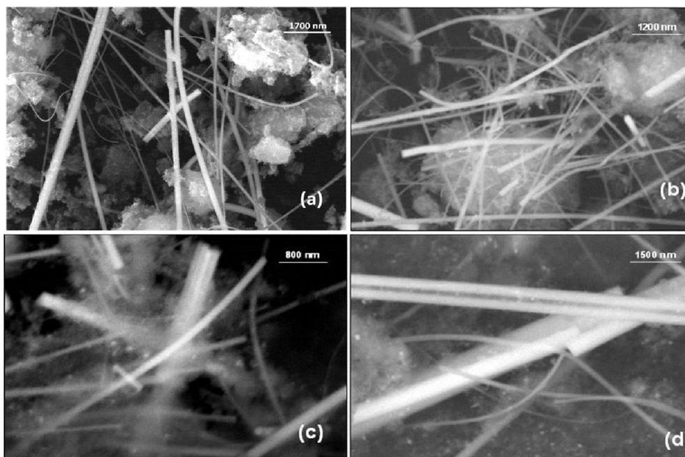
**Fig. 2.** SEM Images of nanorods produced using acetylene and oxygen in the presence of ferrocene as catalyst. (a) Nanorods produced at O/F ratio of 0.6 v/v. (b) Nanorods produced at O/F ratio of 0.8 v/v. (c) Nanorods produced at O/F ratio of 1.0 v/v. (d) Nanorods produced at O/F ratio of 1.2 v/v.
