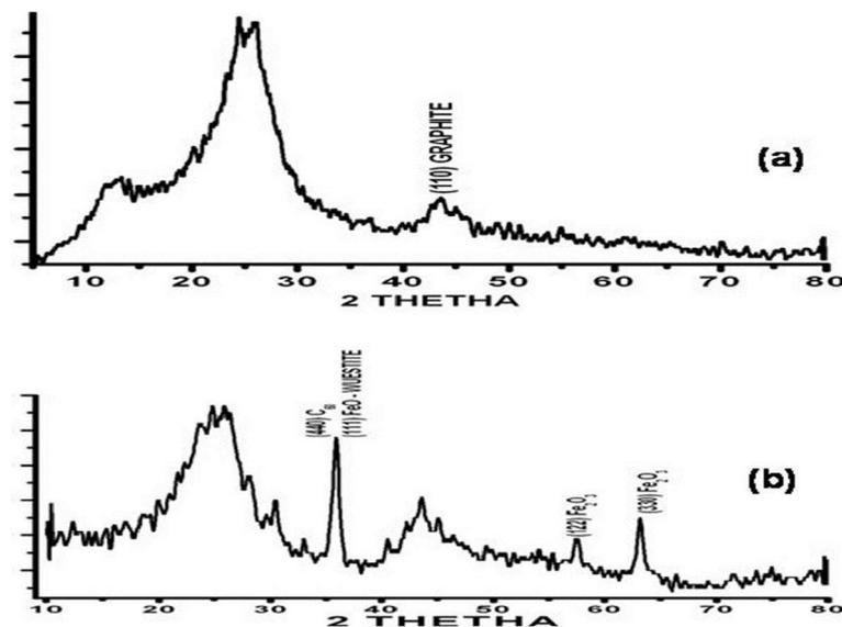
**Fig. 4.** XRD of carbon material produced using acetylene and oxygen. (a) O/F of 0.8 v/v in the absence catalyst. (b) O/F of 0.8 v/v in the presence of catalyst.
