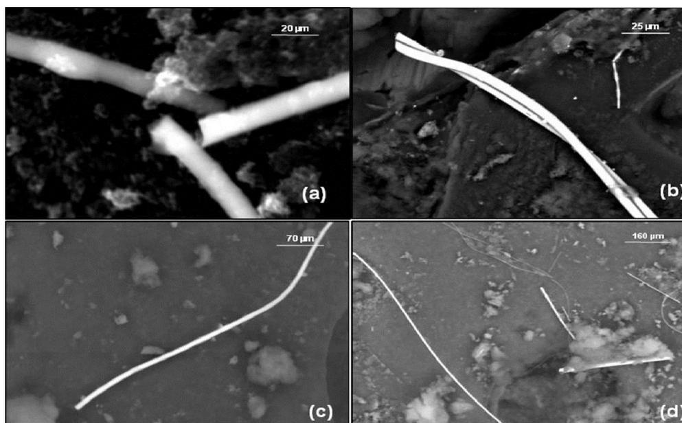
**Fig. 1.** SEM Images of microrods produced using acetylene and oxygen in the absence of catalyst. (a) Microrods produced at O/F ratio of 0.6 v/v. (b) Microrods produced at O/F ratio of 0.8 v/v. (c) Microrods produced at O/F ratio of 1.0 v/v. (d) Microrods produced at O/F ratio of 1.2 v/v.
