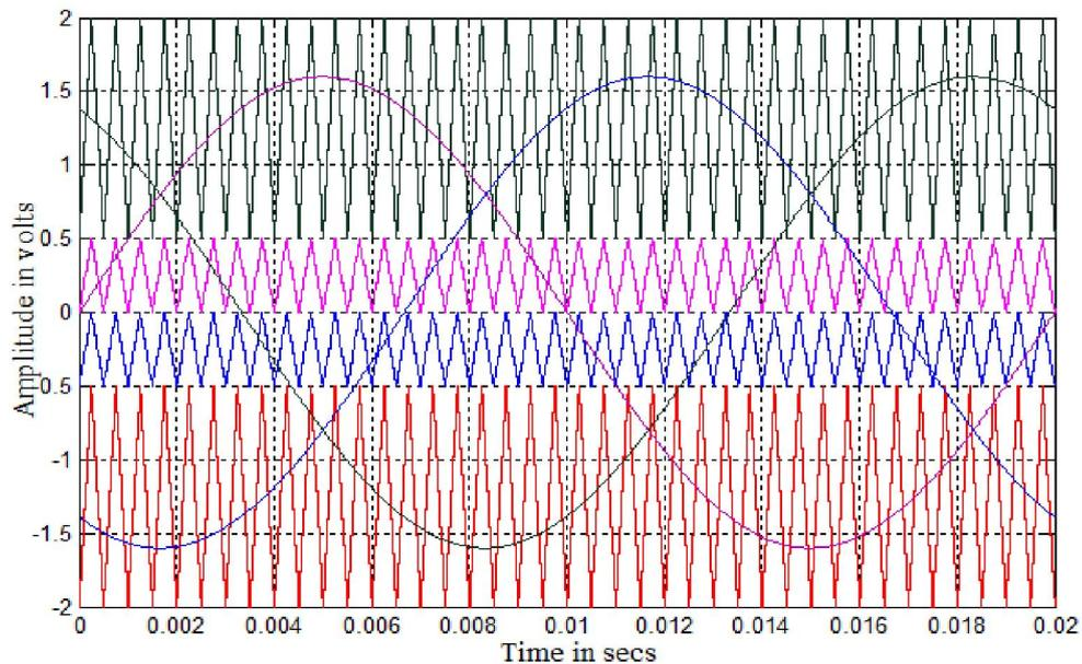
Fig. 3. Modulating and carrier waveforms for VAPDPWM strategy ( $m_a = 0.8$  and  $m_f = 40$ )
