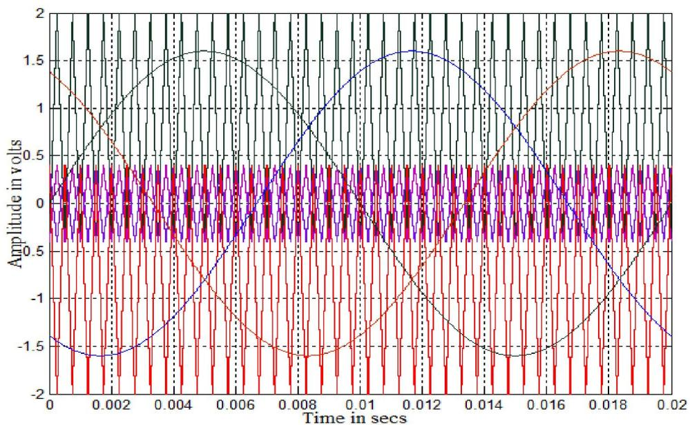
**Fig. 13. Modulating and carrier waveforms for VACOPWM-B strategy ( $m_a = 0.8$  and  $m_f = 40$ )**
