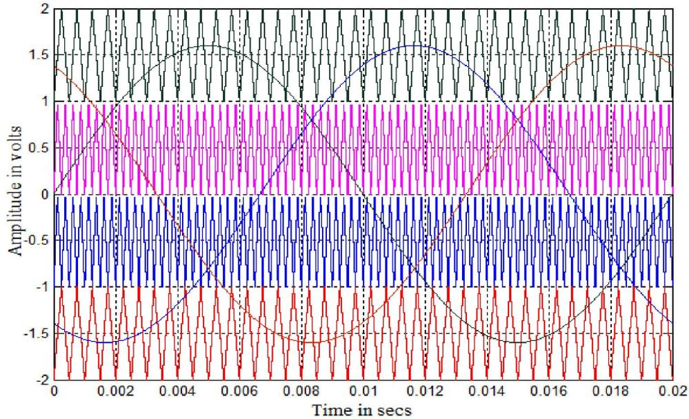
**Fig. 8. Modulating and carrier waveforms for VFPWM strategy ( $m_a = 0.8$  and  $m_f = 40$  for upper switches and  $m_a = 0.8$  and  $m_f = 80$  for intermediate switches)**
