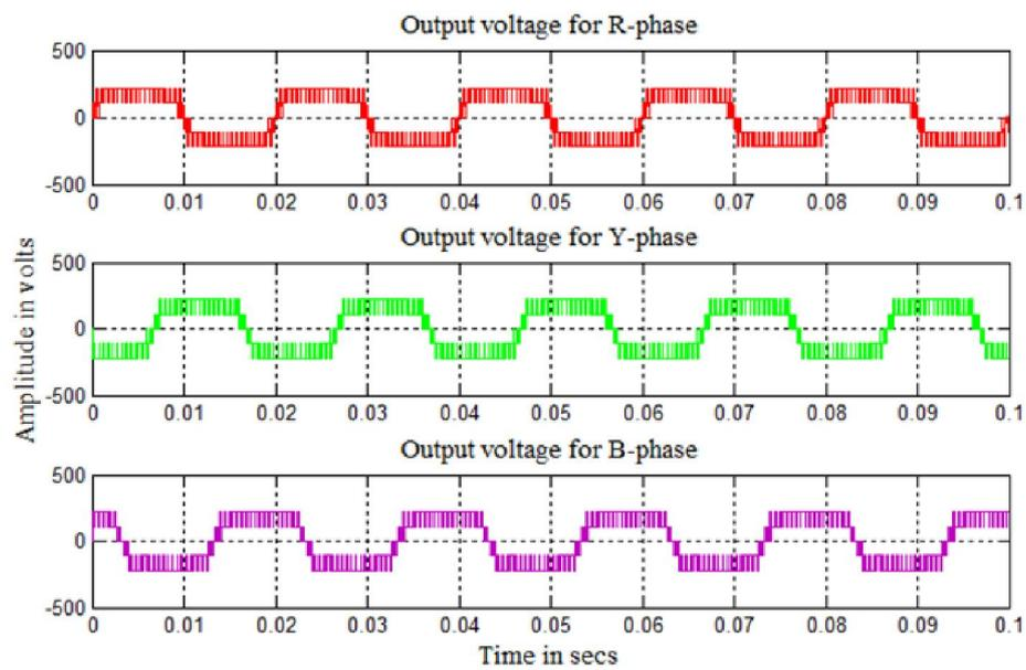
Fig. 20. Simulated output voltage generated by VACOPWM-B technique for R-load
