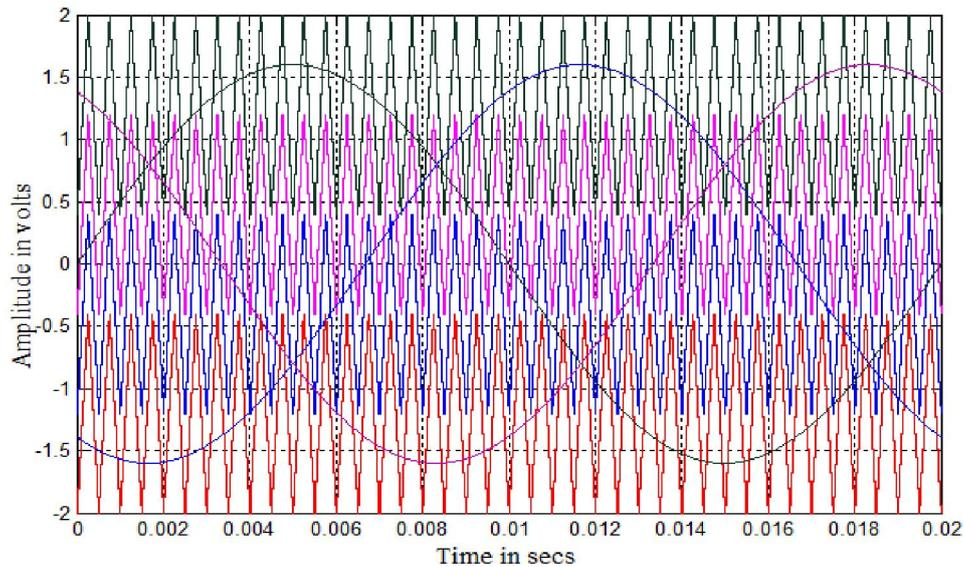
Fig. 10. Modulating and carrier waveforms for COPWM-A strategy ( $m_a = 0.8$  and  $m_f = 40$ )
