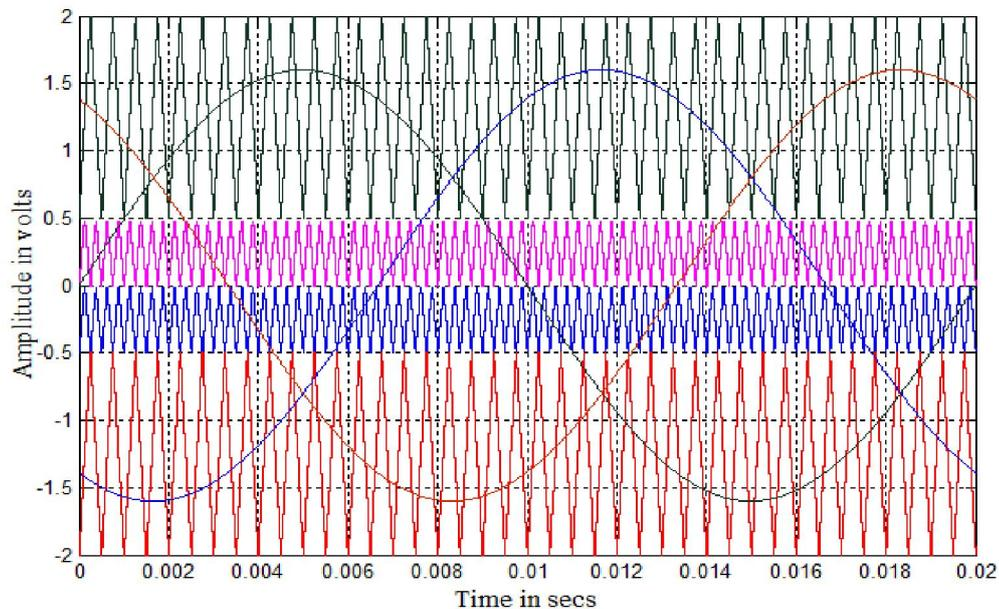
**Fig. 9. Modulating and carrier waveforms for VAVFPWM strategy ( $m_a = 0.8$  and  $m_f = 40$  for upper switches and  $m_a = 0.8$  and  $m_f = 80$  for intermediate switches)**
