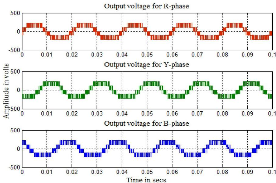
**Fig. 18.** Simulated output voltage generated by COPWM-C technique for R-load
