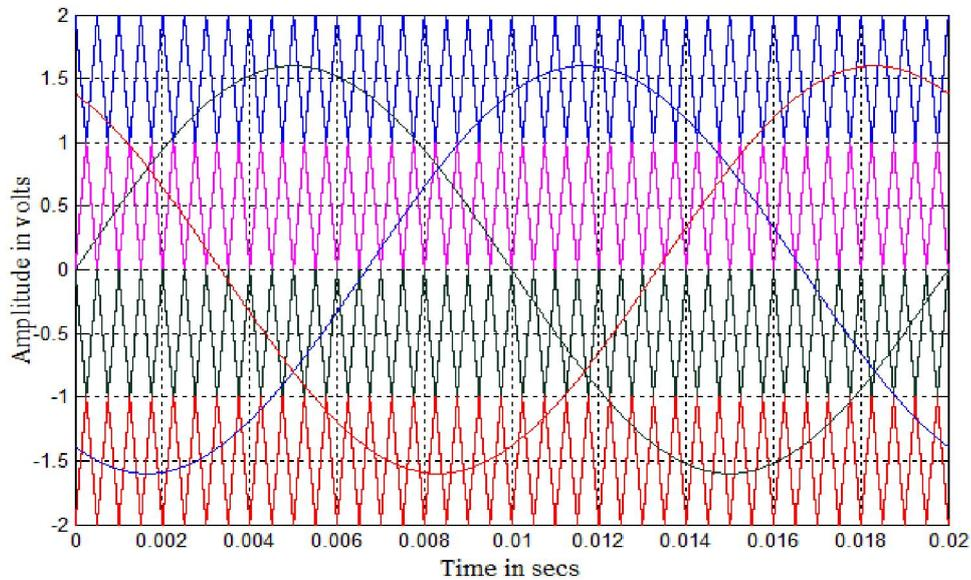
Fig. 6. Modulating and carrier waveforms for APODPWM strategy ( $m_a = 0.8$  and  $m_f = 40$ )
