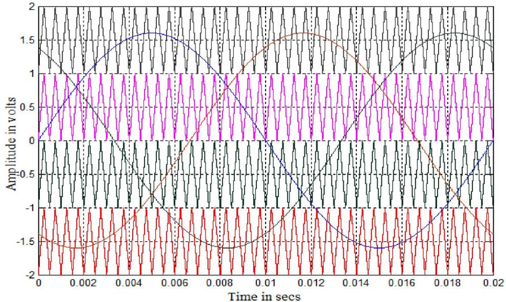
Fig. 2. Modulating and carrier waveforms for PDPWM strategy ( $m_a = 0.8$  and  $m_f = 40$ )
