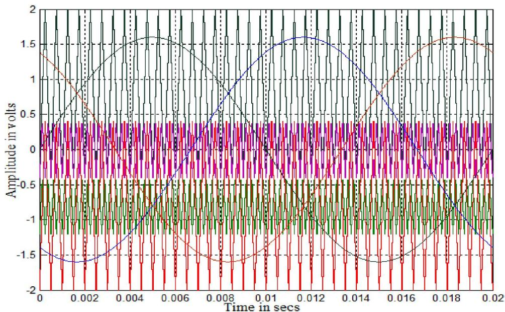
**Fig. 17. Modulating and carrier waveforms for COPWM-D strategy ( $m_a = 0.8$  and  $m_f = 40$  for upper switches and  $m_a = 0.8$  and  $m_f = 80$  for intermediate switches)**
