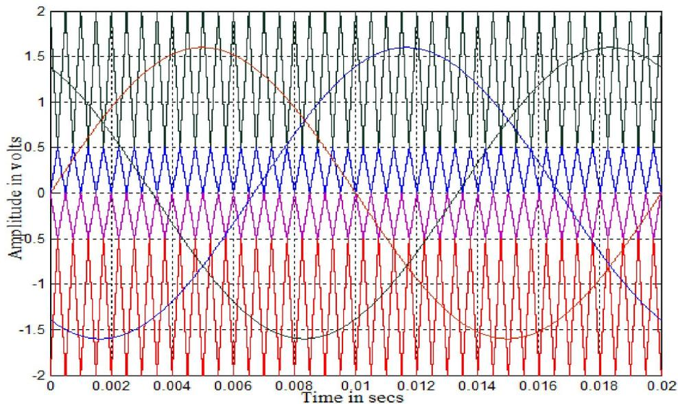
Fig. 7. Modulating and carrier waveforms for VAAPODPWM strategy ( $m_a = 0.8$  and  $m_f = 40$ )
