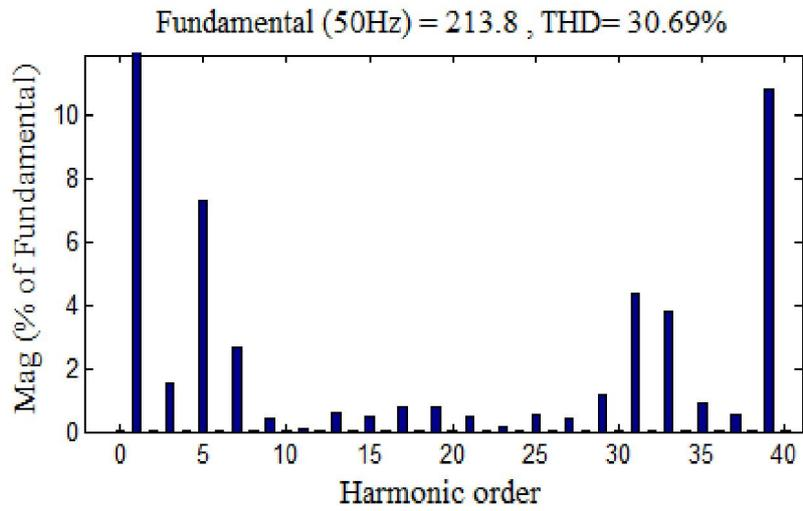
Fig. 22. FFT spectrum for VACOPWM –C technique
