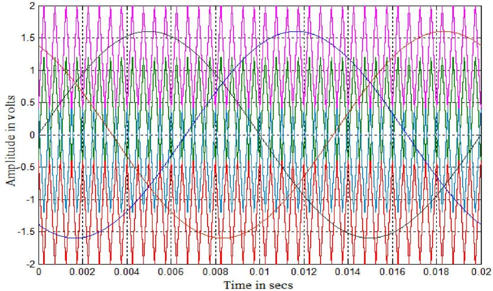
**Fig. 12. Modulating and carrier waveforms for COPWM-B strategy ( $m_a = 0.8$  and  $m_f = 40$ )**
