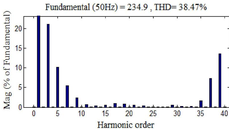
Fig. 23. FFT spectrum for VACOPWM –B technique
