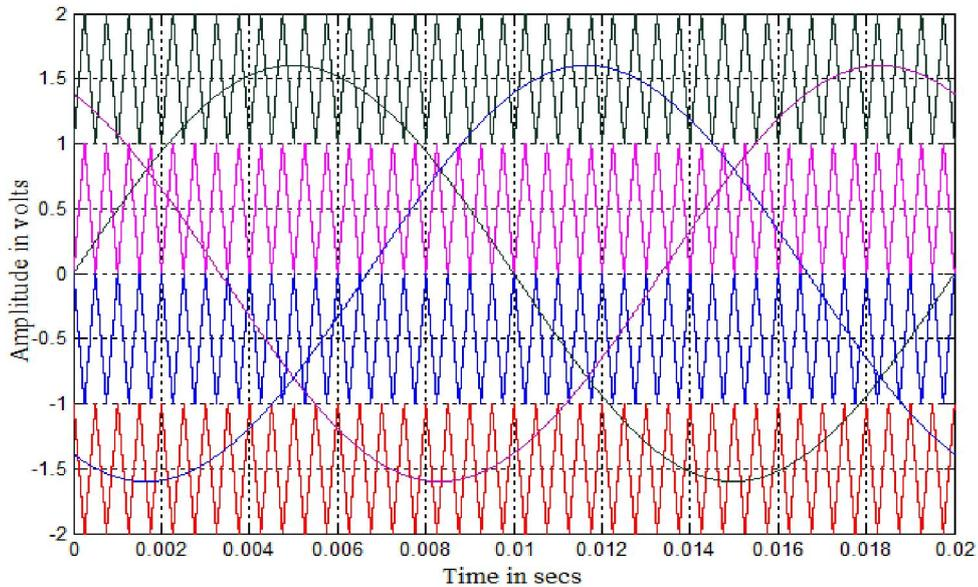
**Fig. 4. Modulating and carrier waveforms for PODPWM strategy ( $m_a = 0.8$  and  $m_f = 40$ )**
