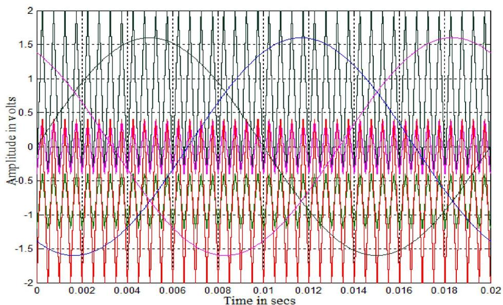
Fig. 11. Modulating and carrier waveforms for VACOPWM-A strategy ( $m_a = 0.8$  and  $m_f = 40$ )
