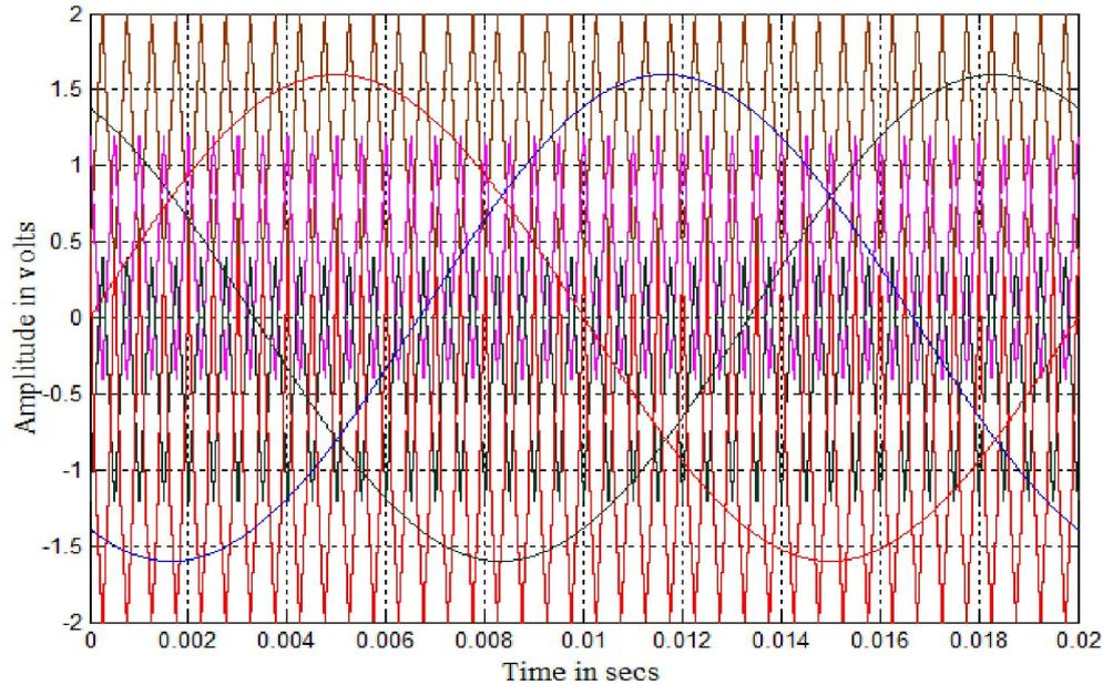
Fig. 14. Modulating and carrier waveforms for COPWM-C strategy ( $m_a = 0.8$  and  $m_f = 40$ )
