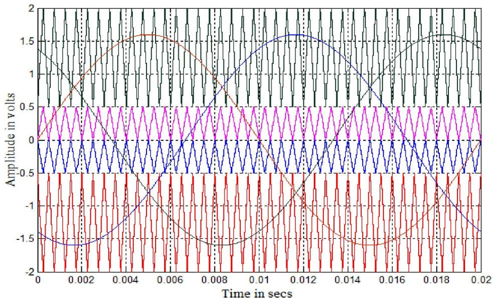
**Fig. 5. Modulating and carrier waveforms for VAPODPWM strategy ( $m_a = 0.8$  and  $m_f = 40$ )**
