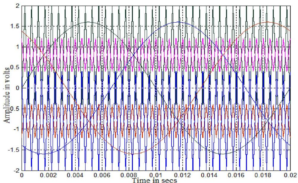
Fig. 15. Modulating and carrier waveforms for VACOPWM-C strategy ( $m_a = 0.8$  and  $m_f = 40$ )
