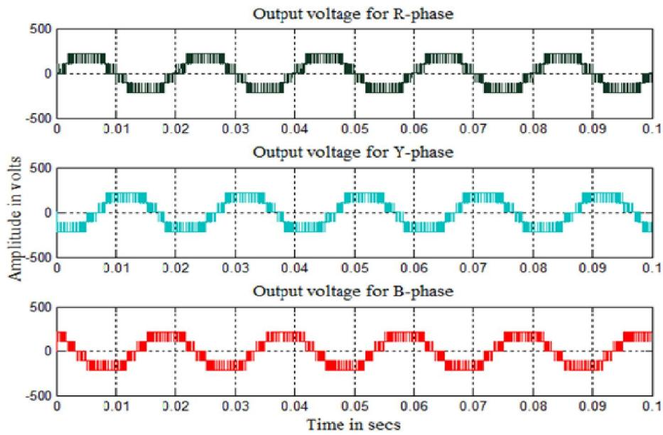
Fig. 19. Simulated output voltage generated by VACOPWM-C technique for R-load
