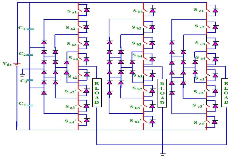
Fig. 1. Three phase five level DCMLI
