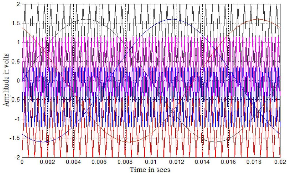
**Fig. 16. Modulating and carrier waveforms for COPWM-D strategy ( $m_a = 0.8$  and  $m_f = 40$  for upper switches and  $m_a = 0.8$  and  $m_f = 80$  for intermediate switches)**
