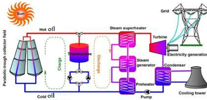
Fig. 3. Mixed-media single tank thermocline system
