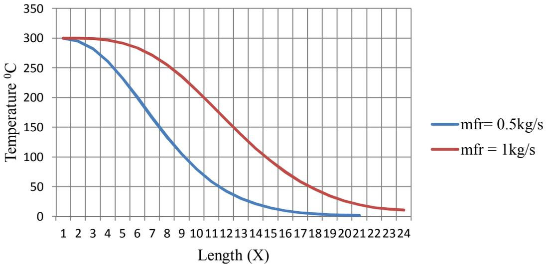
Fig. 11. Temperature distributions on the solid rocks as the mass flow rate changes
