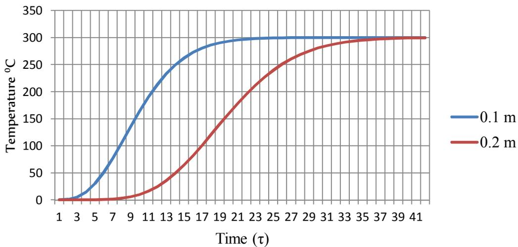
Fig. 5. Temperature distributions on the HTF (oil) at different positions
