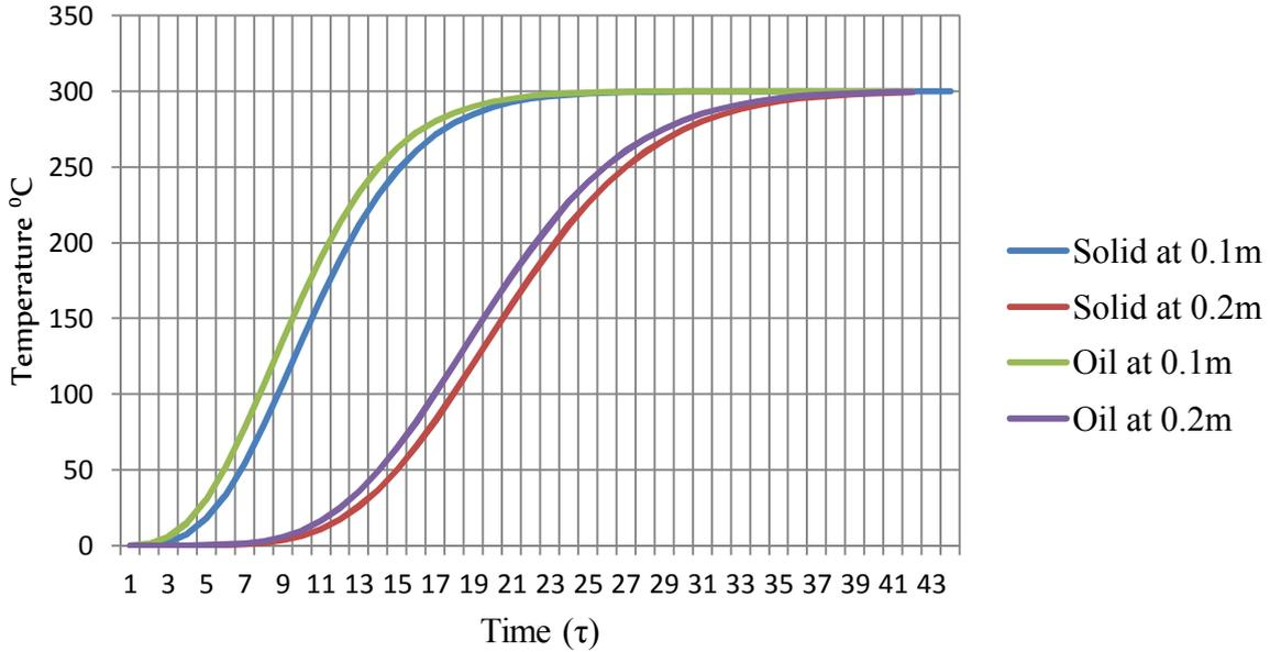
Fig. 10. Temperature distributions on the storage at different positions
