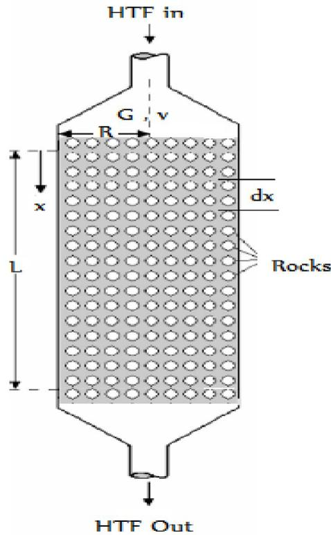
Fig. 4. Model of mixed media thermocline thermal energy storage
