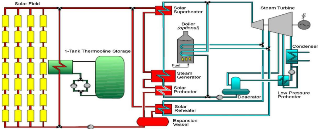
Fig. 1. Single-tank indirect thermocline thermal energy storage [1]
