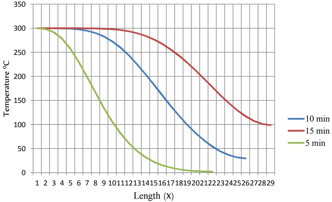
Fig. 6. Temperature distributions on the HTF (oil) in different times
