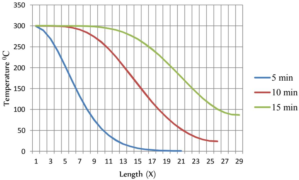
Fig. 7. Temperature distributions on the solid rocks at different times
