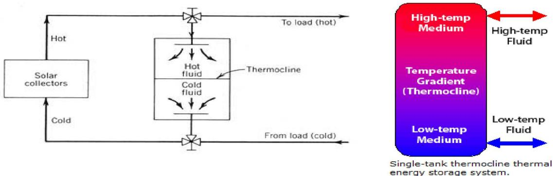
Fig. 2. Thermocline thermal energy storage
