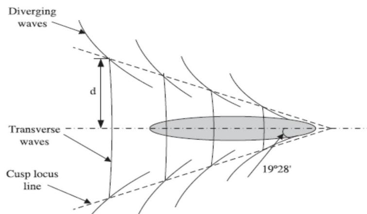
**Fig. 1. Ship generated wave model**
