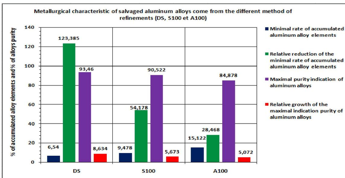
Fig. 1. Metallurgic characteristic according to refining techniques (DS, S100 et A100)
