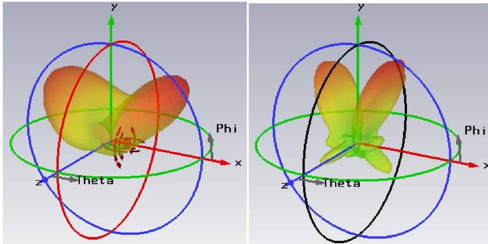
Fig. 4. (a): directivity of antenna for downlink band (b): directivity of antenna for uplink band
