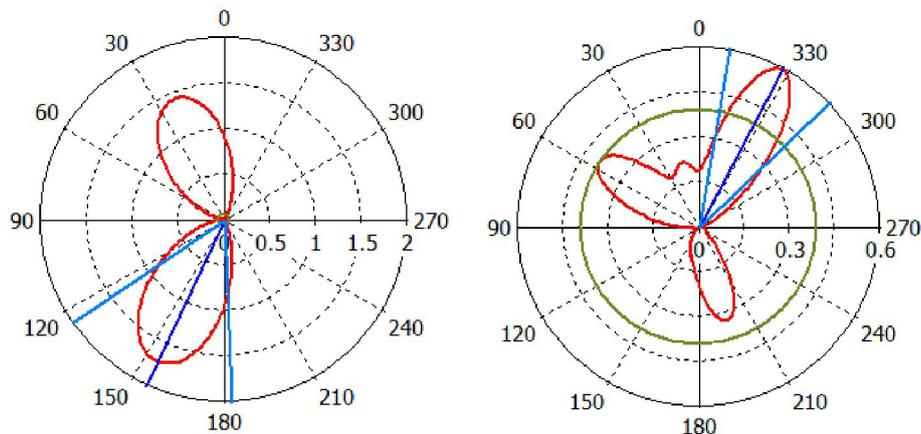
Fig. 5. (a): gain of the proposed antenna for downlink application (b): gain of the proposed antenna for uplink application
