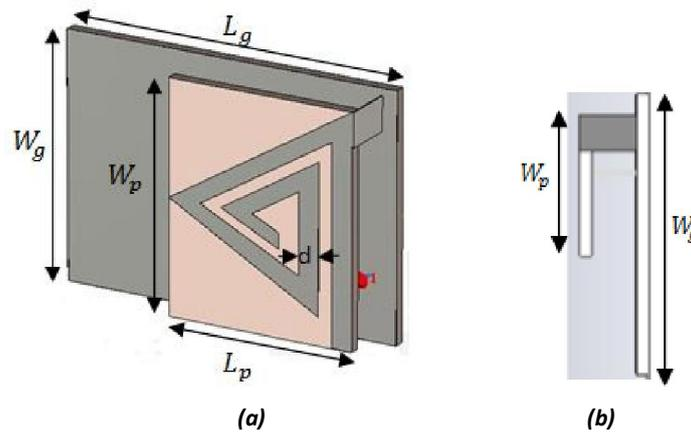
Fig. 2. Proposed triangular Meander – Line Antenna (a) Perspective view, (b) Side view
