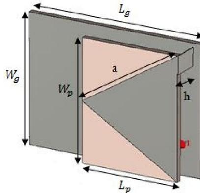
Fig. 1. Triangular PIFA Antenna
