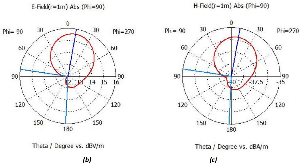
Fig. 4. (a) 3-Dimensional Radiation Pattern, (b) E-field Pattern, (c) H-field Pattern
