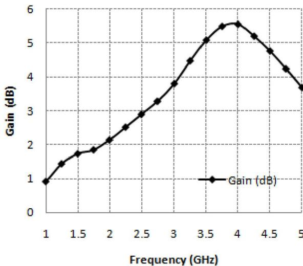
Fig. 5. Simulated Peak Gain of the Triangular Meander-Line PIFA antenna
