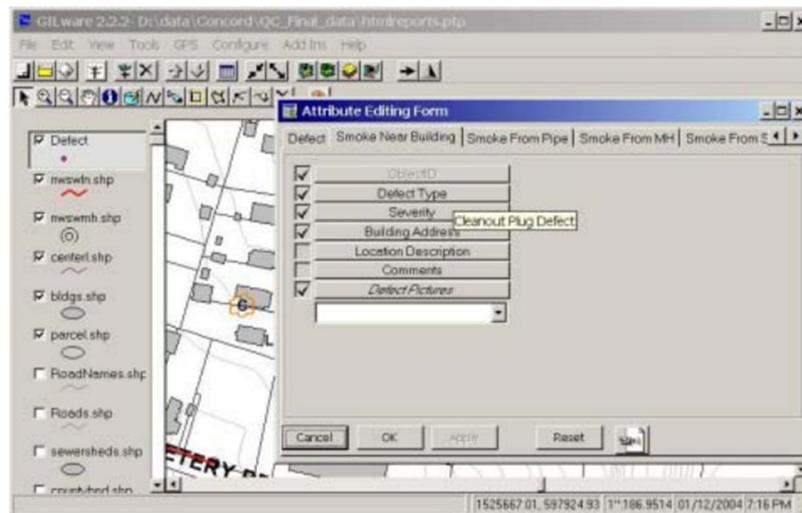
**Fig. 6. A GIS application that allows field crews to attribute defects with both location and tabular data. Also, the application relates one or more digital pictures to the defect at the time of capture**
