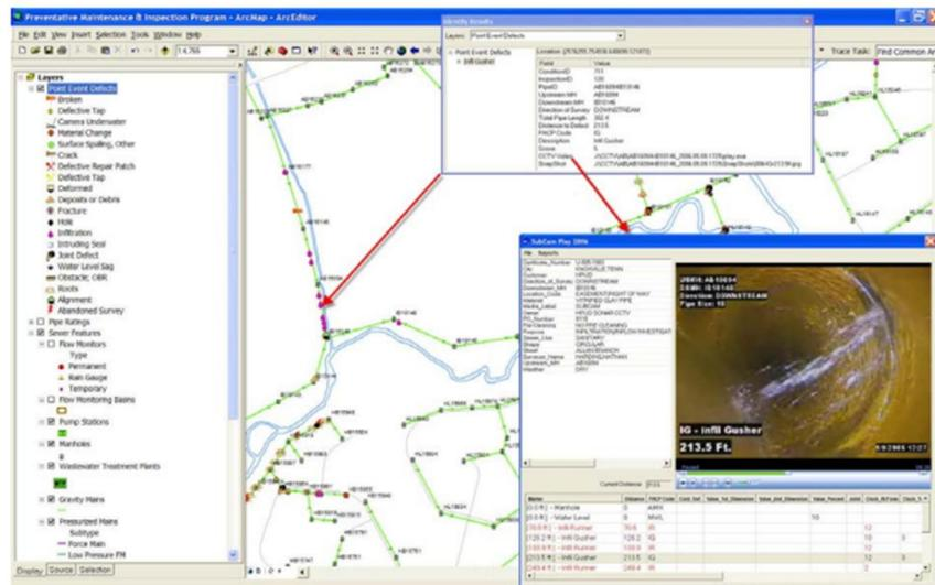
**Fig. 5. TV inspection footage is hyperlinked for multimedia viewing within the mapping software**
