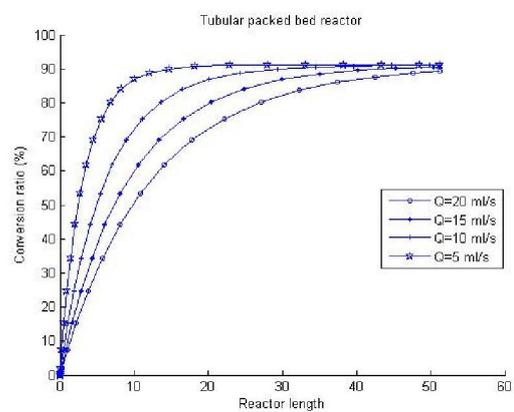
Fig. 6. Effect of flow rate on the conversion of SO<sub>2</sub> along the packed bed (3%SO<sub>2</sub>, T=773K)
