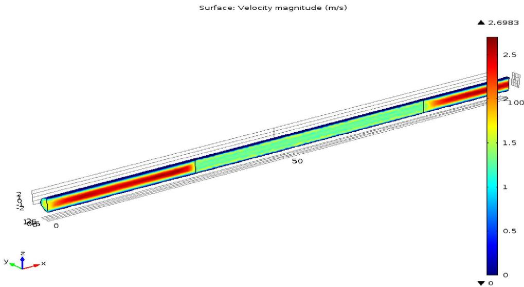
**Fig. 7. Magnitude of the velocity field in the free and porous reactor domains**
