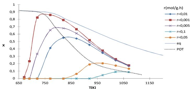
Fig. 2. Conversion of SO<sub>2</sub> versus temperature at various reaction rates
