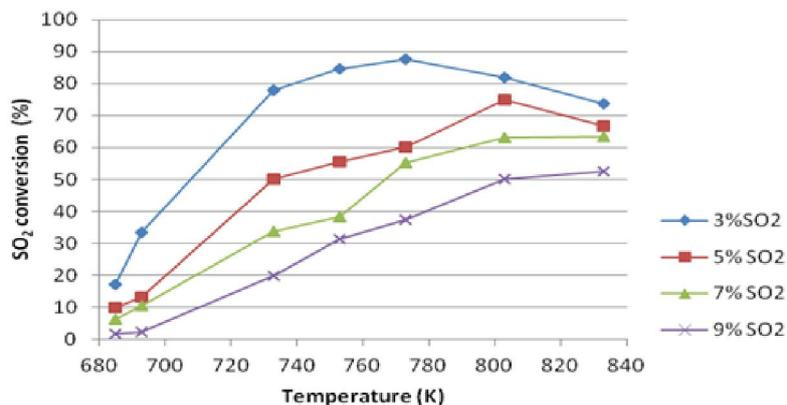
Fig. 1. Influence of temperature on conversion rate for various inlet SO<sub>2</sub> contents
