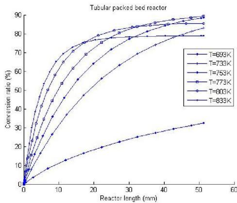
Fig. 5. Conversion of SO<sub>2</sub> along the packed bed (3%SO<sub>2</sub>, Q=20ml/s)
