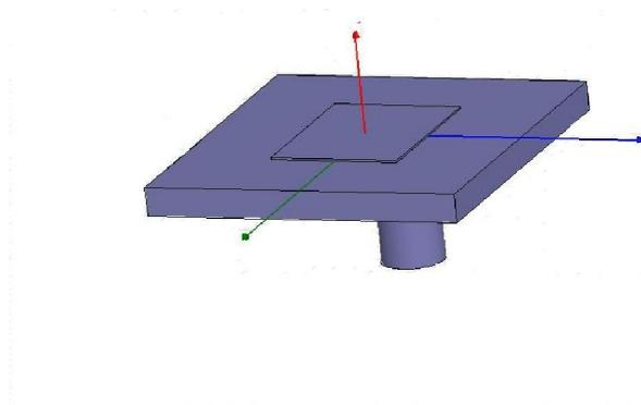
**Fig. 1. Rectangular Patch Antenna**
