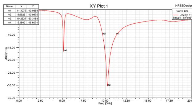
Fig. 5. Return loss of an antenna with Metamaterial structure
