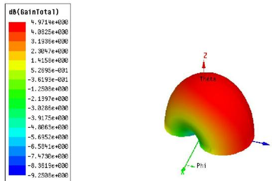
Fig. 10. Gain of an antenna without Metamaterial structure
