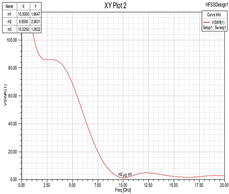
Fig. 8. VSWR of an antenna without Metamaterial structure
