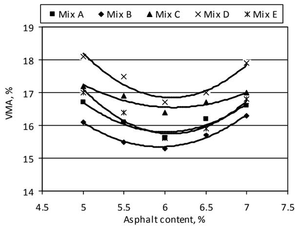
Fig. 4. Voids in mineral aggregate of asphalt-concrete with different filler materials
