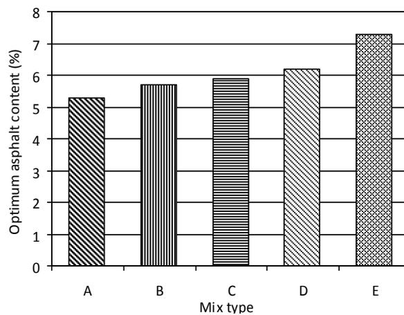
Fig. 8. Optimum asphalt content of asphalt-concrete with different filler materials
