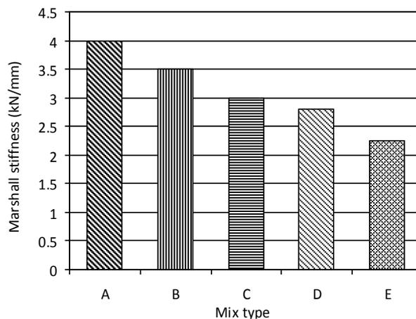
Fig. 9. Marshall stiffness of asphalt-concrete with different filler materials
