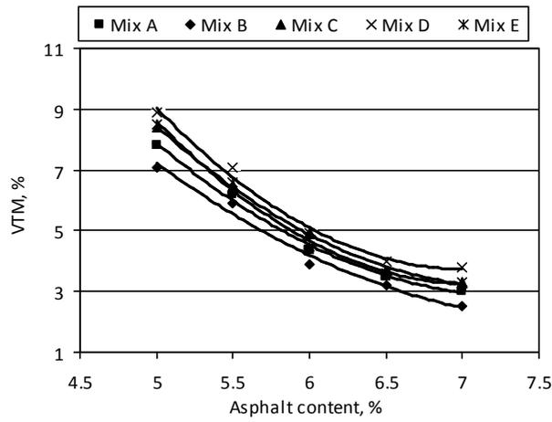
Fig. 3. Voids in total mix of asphalt-concrete with different filler materials
