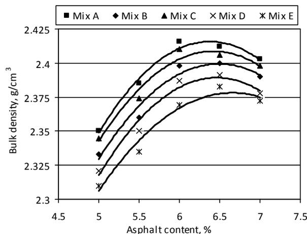
Fig. 2. Bulk density of asphalt-concrete with different filler materials
