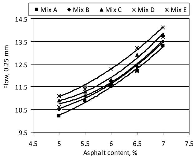
Fig. 7. Flow value of asphalt-concrete with different filler materials
