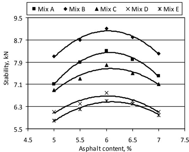
Fig. 6. Marshall stability of asphalt-concrete with different filler materials
