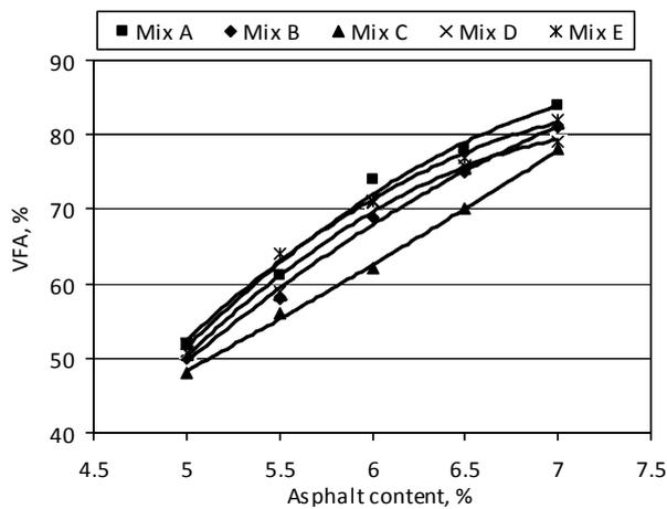
Fig. 5. Voids filled with asphalt of asphalt-concrete with different filler materials
