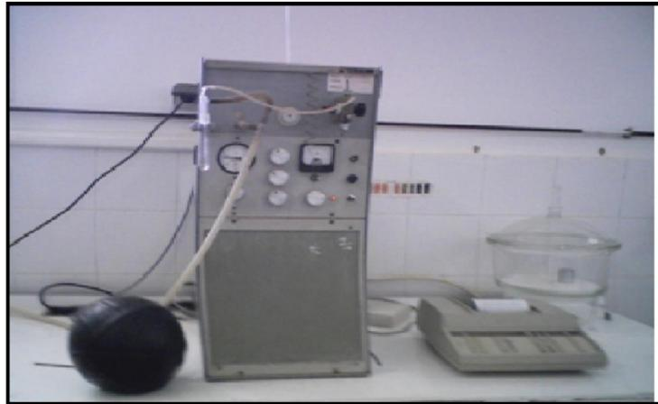
**Fig. 2. The chromatography for the estimation of the composition of gas**
