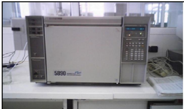
**Fig. 3. The chromatography for the estimation of the calorific values**
