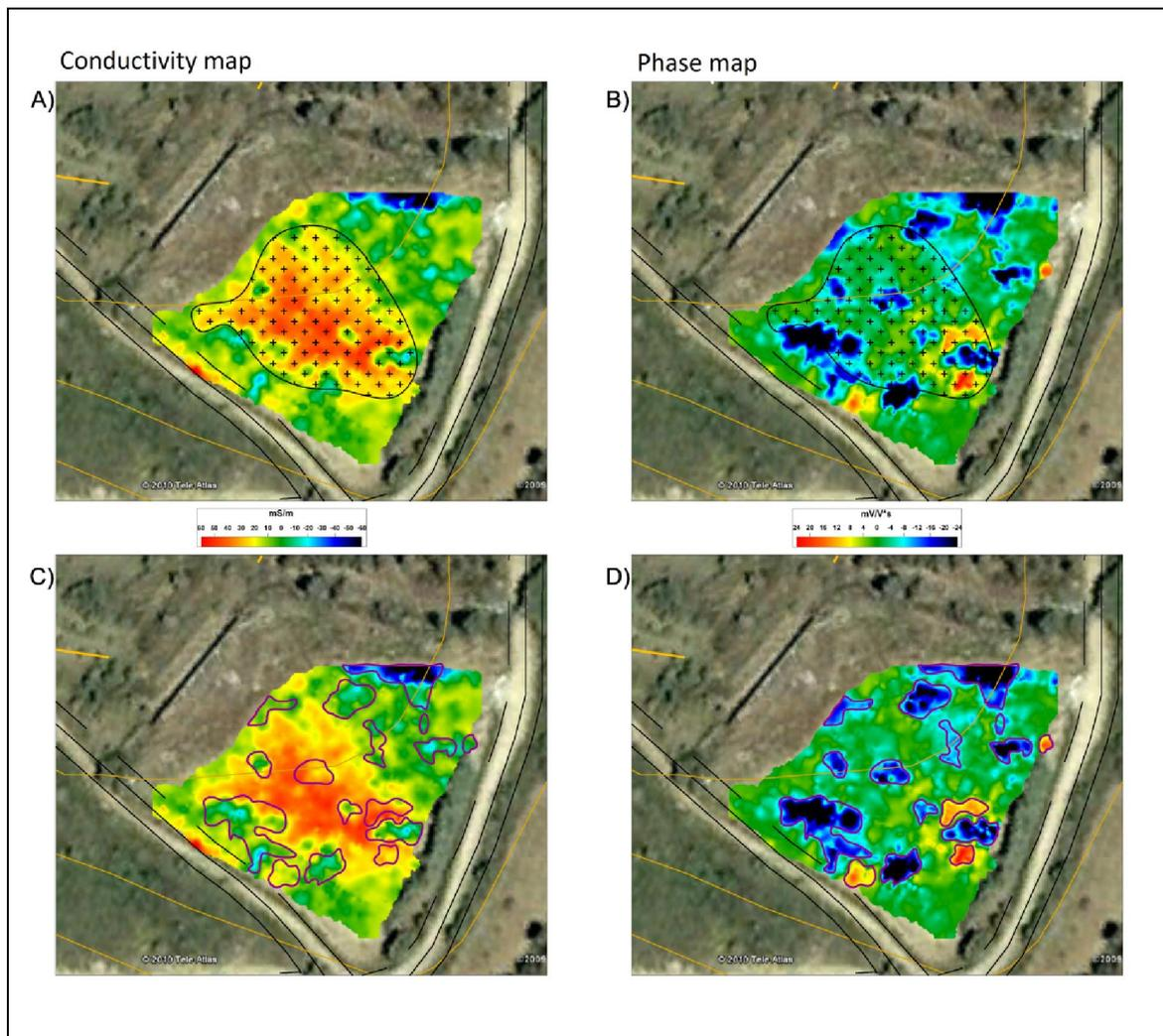
**Fig. 4. FDEM results, A,C) Apparent conductivity maps, B,D) phase response maps**
