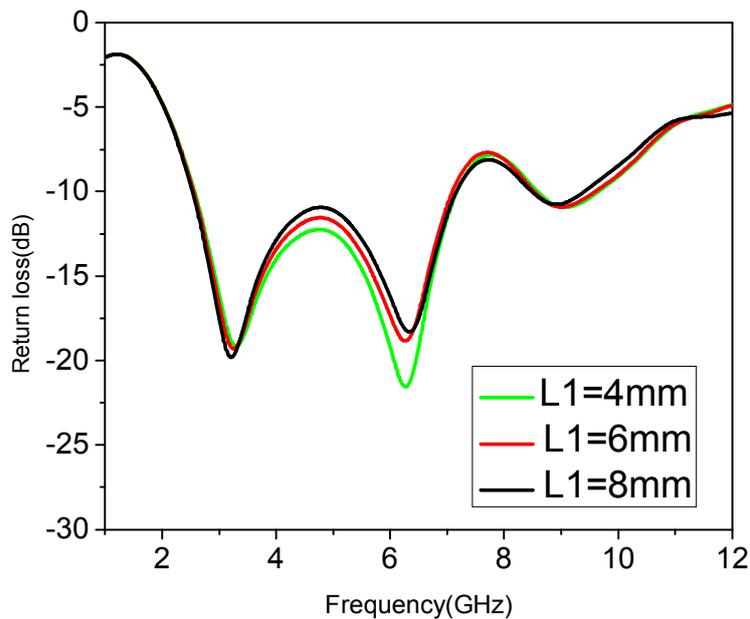
**Fig. 4.** The return loss of the antenna functions ( $L_1$ )
