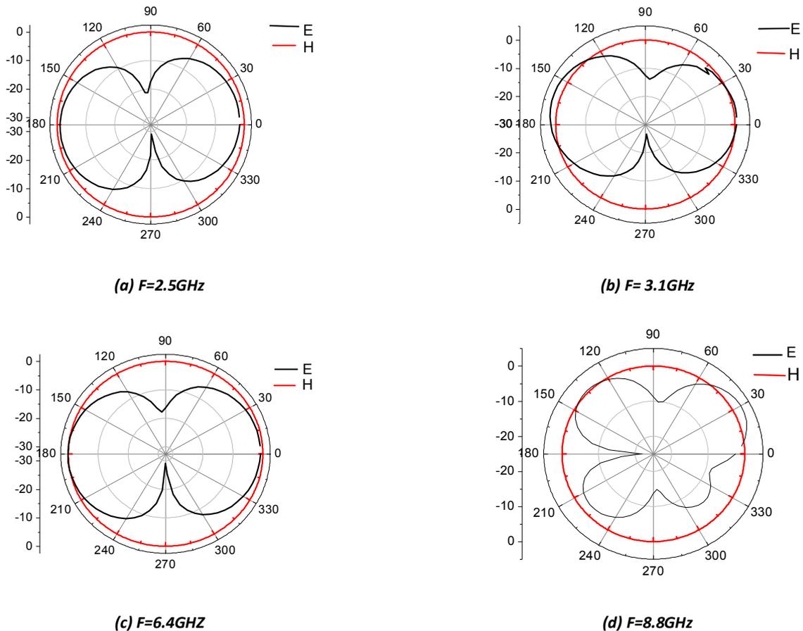
Fig. 7. Radiation pattern of the antenna, (a)  $f = 2.5\text{GHz}$ , (b)  $f = 3.1\text{GHz}$ , (c)  $f = 6.4\text{GHz}$  and (d)  $8.8\text{GHz}$
