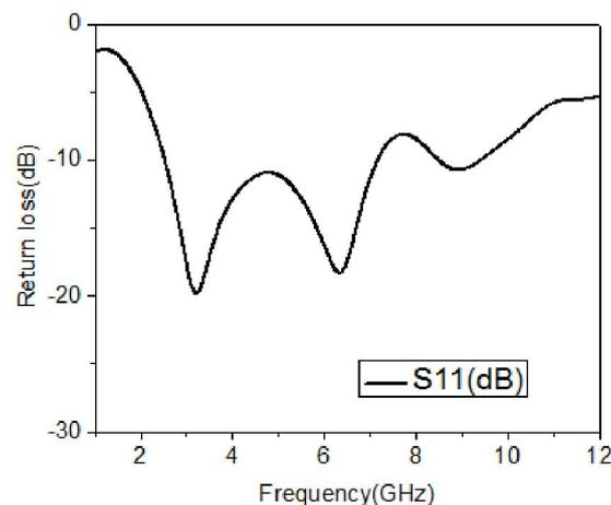
Fig. 2. The return loss  $S_{11}$  of the proposed antenna at  $L_1 = 8\text{mm}$ ,  $W_1 = 9\text{mm}$ ,  $L_g = 10\text{mm}$
