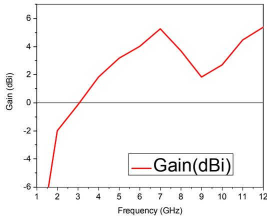
Fig. 6. gain of the proposed antenna
