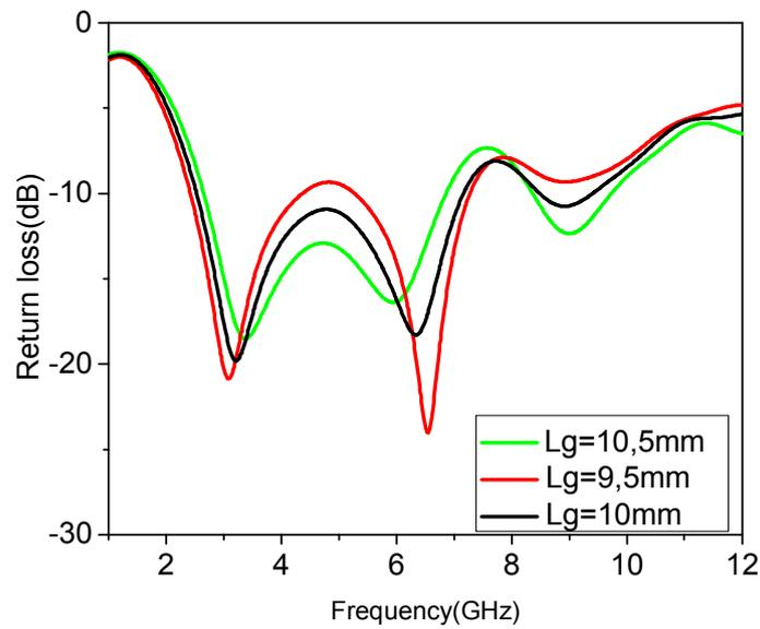
Fig. 5. The reflection coefficients of the antenna functions (Lg)
