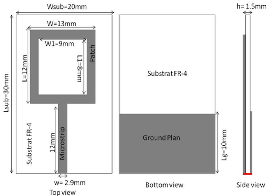
Fig. 1. Geometry of the proposed antenna
