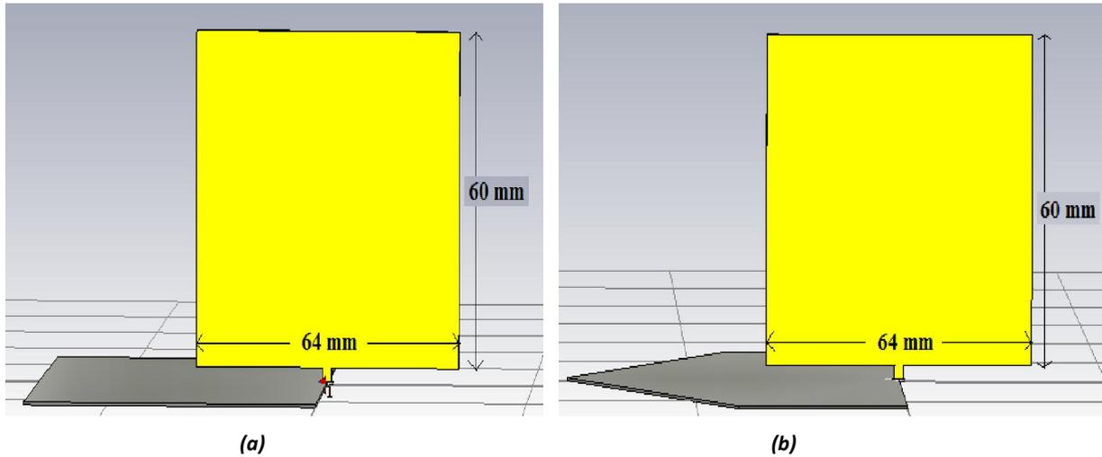
**Fig. 2.** Geometry of the proposed planar rectangular monopole antenna on CST (a) with one sided half rectangular ground plane (b) one side half hexagon ground plane.
