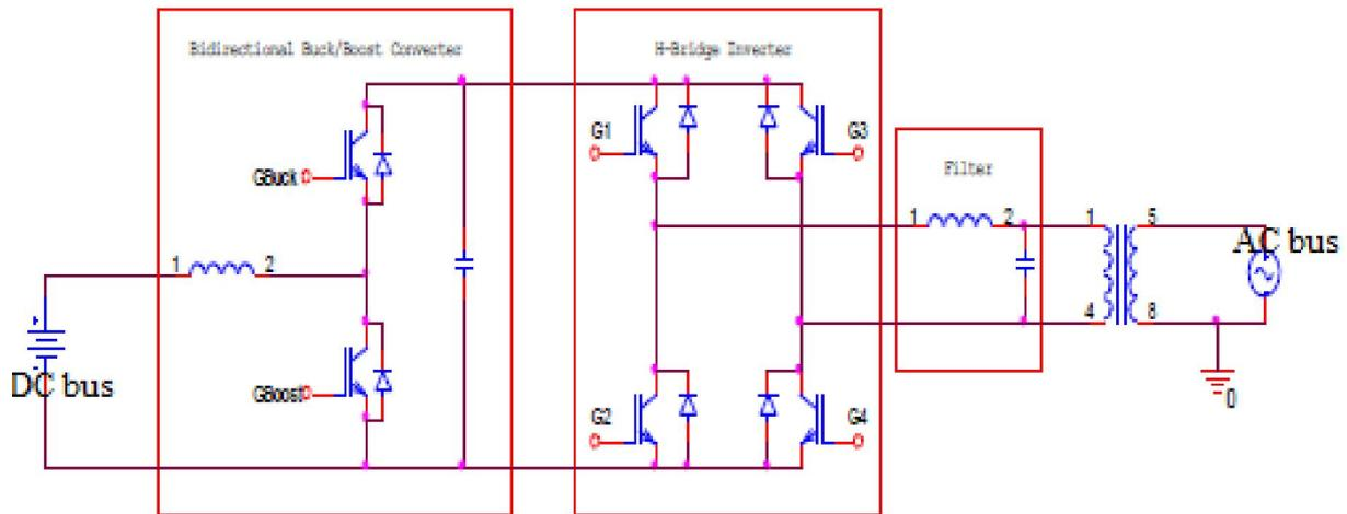
**Fig. 8. Circuit diagram of Bi-directional Inverter**
