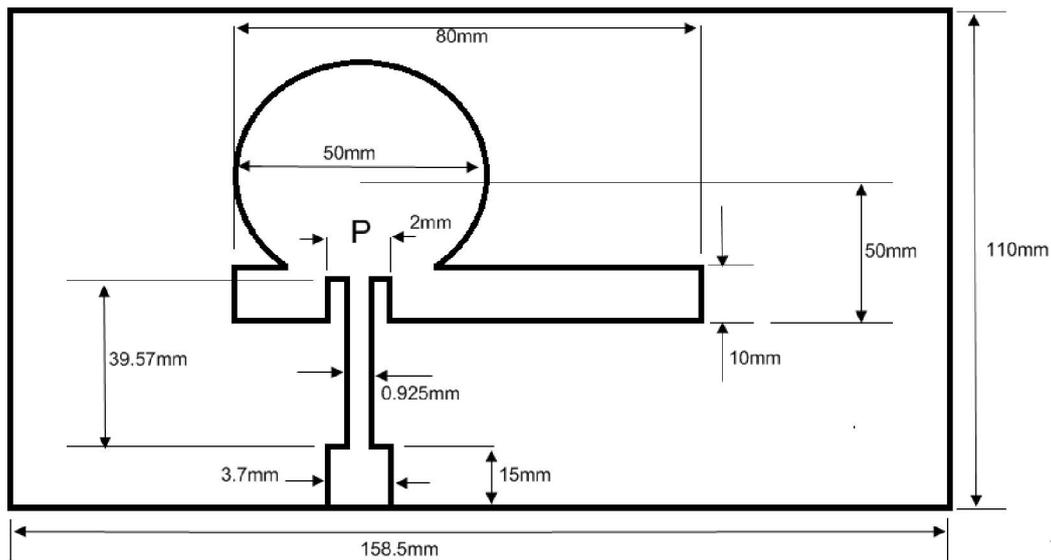
Fig. 1. Geometry of the P-shaped wearable patch antenna
