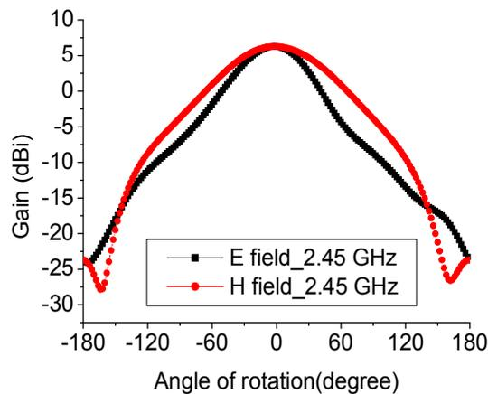
Fig. 2. Simulated result of radiation pattern at 2.45GHz
