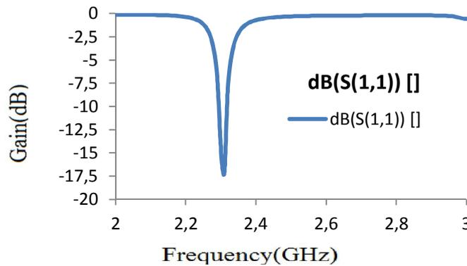
Fig. 4. Simulated result of RL. at 2.45GHz
