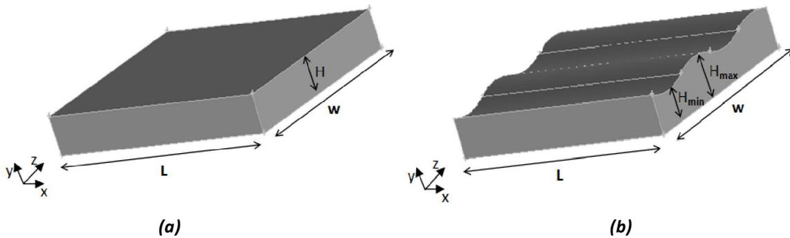
Fig. 1. Studied geometries: (a) flat plate channel, (b) channel with sinusoidal upper plate
