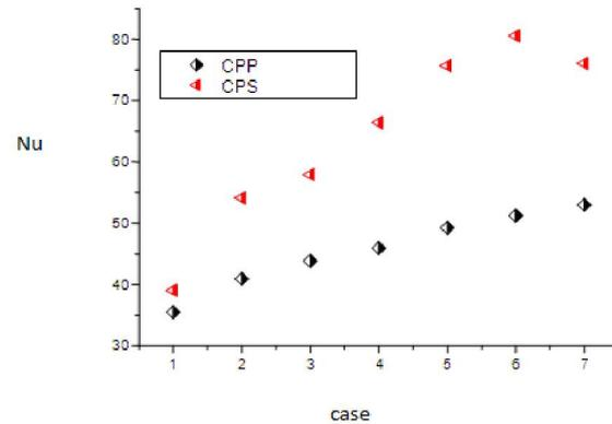
Fig. 9. Comparison of the average convection coefficient for the two types of channels
