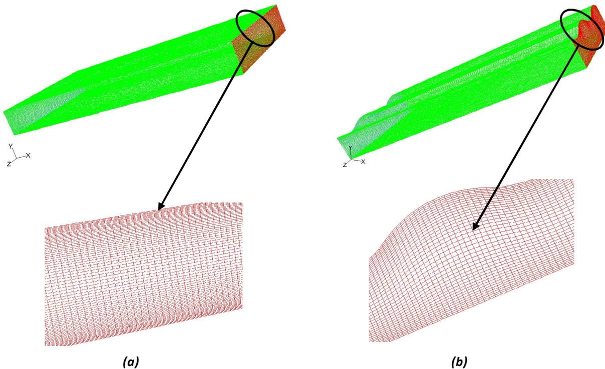
Fig. 3. Mesh geometries studied, (a) channel flat plate, (b) channel with sinusoidal upper plate
