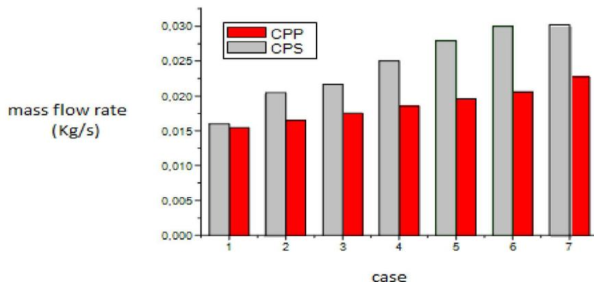
Fig. 8. Comparison of mass flow rates for both channels CPP (channel with flat plates) and CPS (channel sinusoidal plate)
