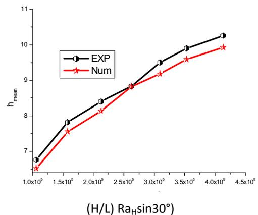
Fig. 6. Comparison of experimental and numerical average coefficient of convection
