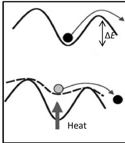
Fig. 5. The mechanism of barrier energy barrier decreases caused by the effect of heat addition (a). barrier energy without the help of heat, (b) barrier energy during heating process
