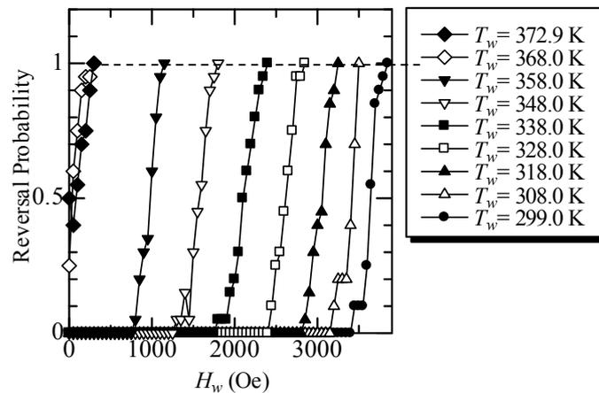
Fig. 3. The likelihood of magnetization reversal against the inductive field on  $K_I = 4.5 \times 10^5 \text{ erg/cm}^3$ ,  $4\pi M_s = 2100 \text{ G}$  with several variances of temperature of writing ( $T_w$ )
