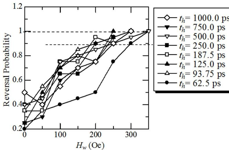
Fig. 6. Profile of  $H_w$  against the likelihood of reversal towards  $K_{\perp} = 4.5 \times 10^5 \text{ erg/cm}^3$ ,  $4\pi M_s = 2100 \text{ G}$  on variances of heating time ( $t_h$ )
