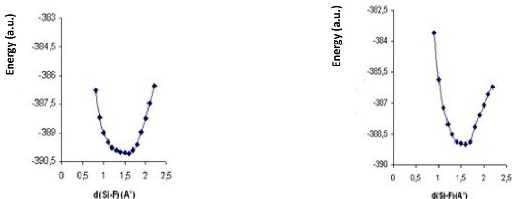
Fig. 3. Energy as a function of equilibrium distance of the Si-F bond (HF and DFT respectively)
