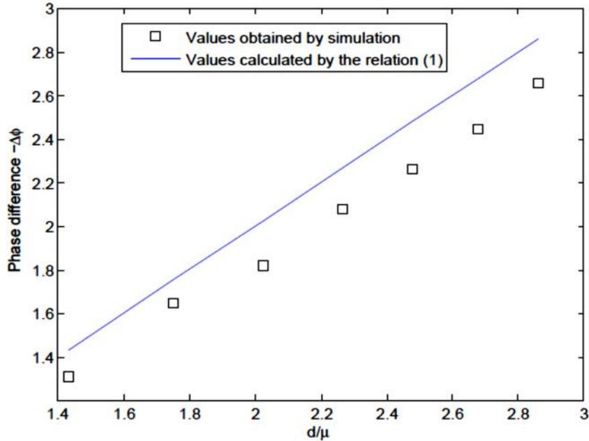
Fig. 2-a: Variation of phase difference opposite  $-\Delta\phi$  versus  $d/\mu$ , Case of PMMA, Maximal gap = 0.2354 rad
