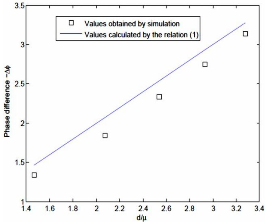
Fig. 2-b: Variation of phase difference opposite  $-\Delta\phi$  versus  $d/\mu$ , Case of polypropylene (PP), Maximal gap = 0.2298 rad
