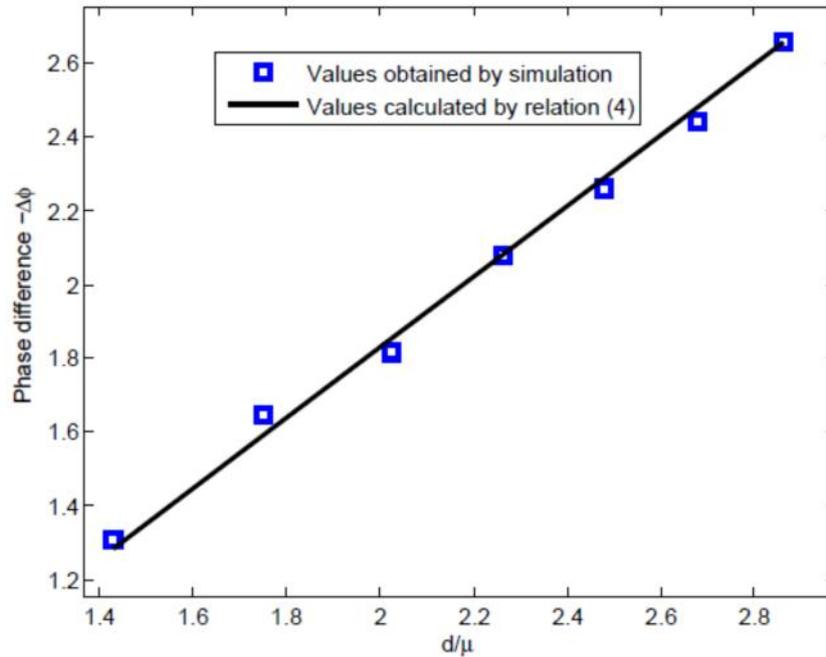
**Fig. 3-a: Results of the proposed model for PMMA sample, Maximal gap = 0.0541 rad.**
